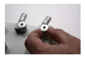
TO INSERT A STRING, TURN THE THUMB WHEEL COUNTER-CLOCKWISE JUST A FEW FULL TURNS TO LOOSEN UP THE MECHANISM. FYI - IF YOU TURN IT TO MUCH, THE WHEEL WILL COME OFF AND A PIN WILL FALL OUT. IF SO, SIMPLY REPLACE THE PIN AND THEN THE WHEEL.
