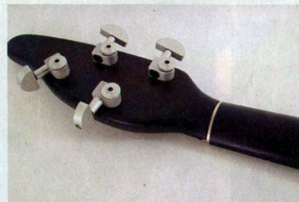
Locking tuners like these Sperzels are more common on tremolo-equipped guitars. The knob on the back of the tuning machines locks the string in place on the post, eliminating the need for multiple winds around the post.
